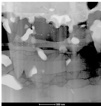
TEM image of the fins in the area of scale and base material, nickel superalloy 718Plus.
