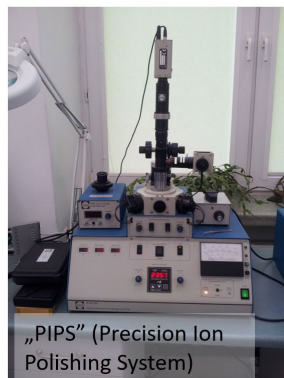
Fig.7. TEM specimen preparation final thinning, ion milling
