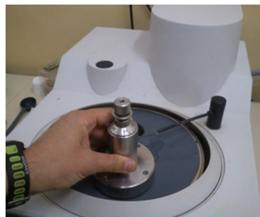
Grinding and polishing to a slice of < 0.1 mm thickness
