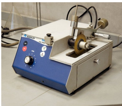
Sawing a slice of about 1 mm thickness
