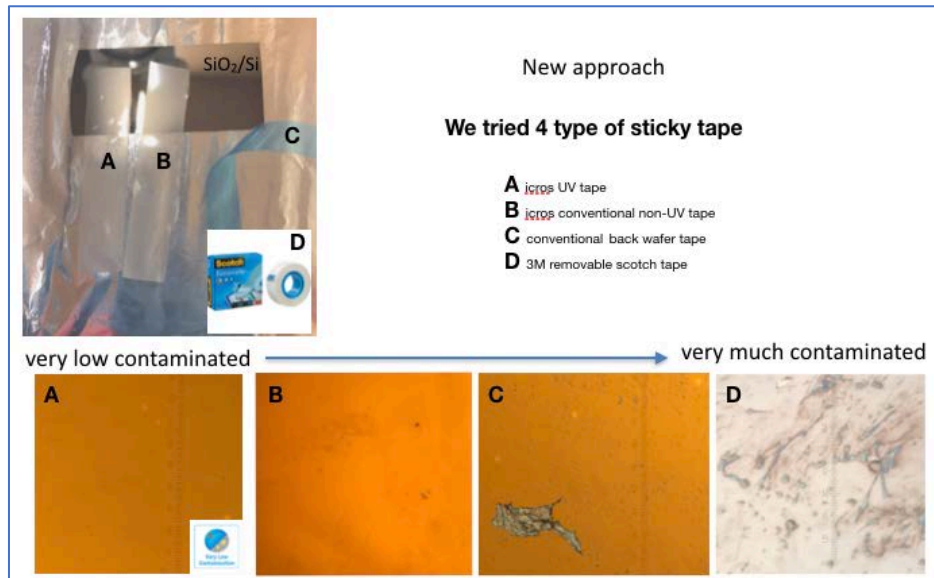
Figure 16. Comparison of Si wafer surface after layer transfer by different kind of sticky tape. From the comparison, it is apparent that the one transferred with the ultraclean icros UV tape is the cleanest
