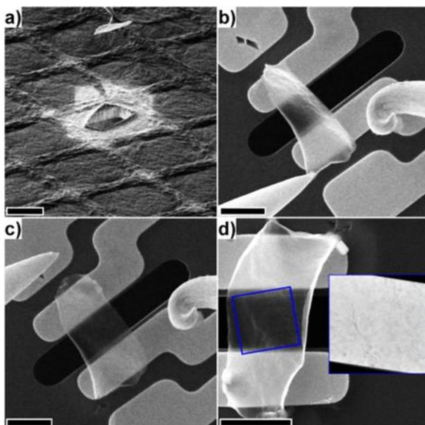
Figure 5. FIB-assisted GO sample preparation. (a) FIB image of a GO piece taken out with a micro-needle from a continuous film on a Cu grid. SEM image of (b) approaching and (c) connected GO piece while
