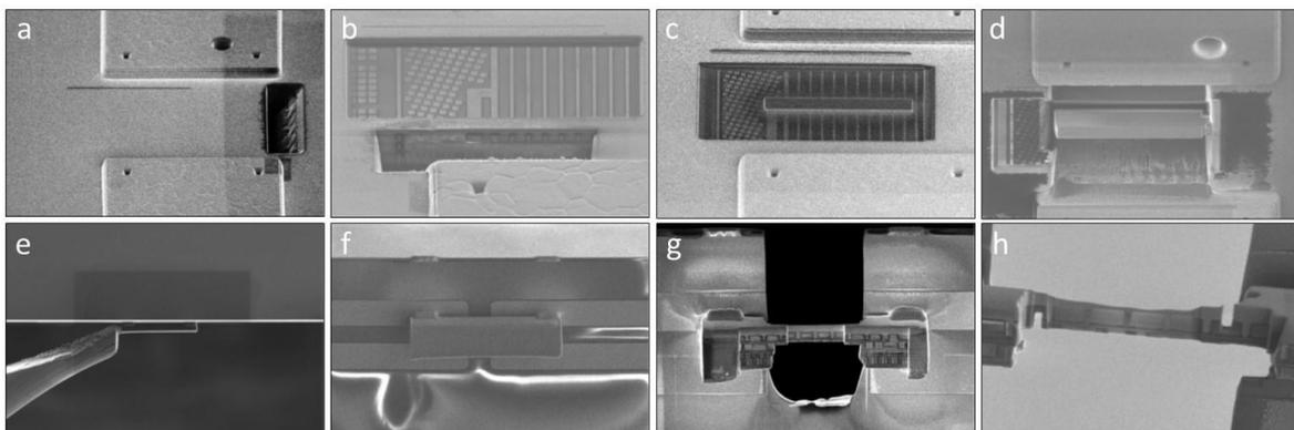
*Figure 1. FIB preparation of specimen-device for in-situ biasing and operando experiments: (a) sample grounding & electrode connections; (b) Cu connects visible after FIB processing; (c) protective Pt layer; (d) sample pre lift-out; (e) sample welding to dedicated TEM grid; (f) chunk welded on TEM grid; (g) TEM grid membrane milling and vacuum area for EH reference wave; (h) final thinning and electrodes separation.*
