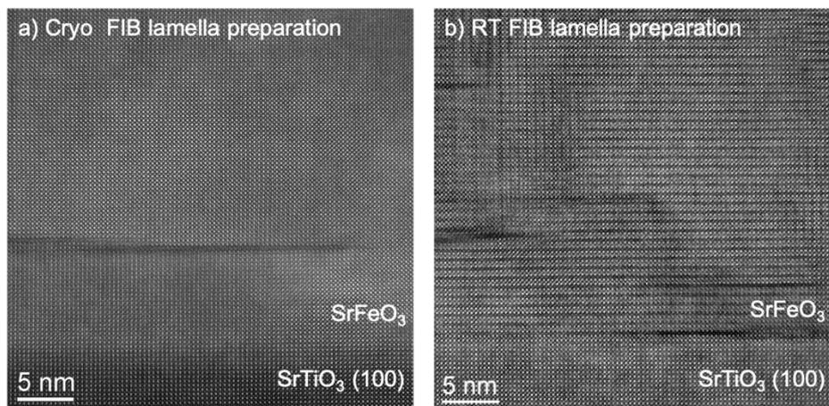
*Figure 4. Cryogenic preparation of TEM lamella of beam sensitive  $\text{SrFeO}_{3-\delta}$ . a) HAADF-STEM image of a cross-sectional TEM lamella of a  $\text{SrFeO}_3$  thin film prepared using the protocol described in this report. b) HAADF-STEM image of the same system prepared by standard RT Ga FIB.*
