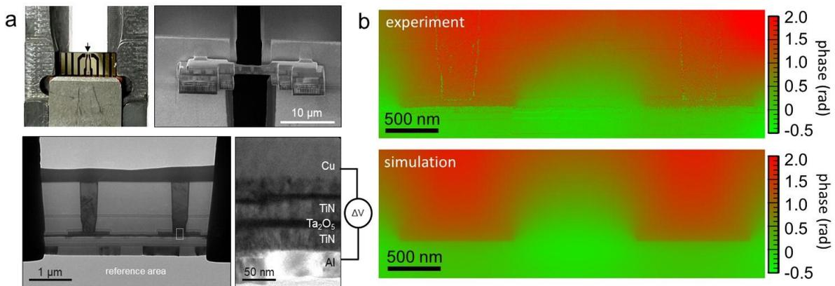
Figure 2. Operando electron holography on working nanocapacitor device: (a) sample-device on chip inserted in in-situ biasing holder (Hummingbird) and progressive enlargements showing active area; (b) experimental electron hologram phase map due to biasing; (c) corresponding simulated phase map from finite-element modelling.
