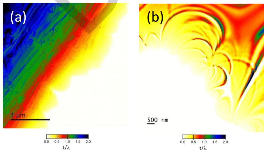
Figure 1.  $t/\lambda$  thickness maps of two GaN samples prepared with an optimized wedge polishing procedure followed by Ar ion milling in (a) and mechanical dimpling followed by ion milling in (b).
