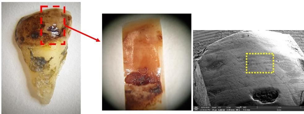
Figure 3: FIB sample preparation of dental pathologies. Presented is a diseased human tooth. FIB sample shown in Figure 4 was prepared from an area marked with the yellow square (right image).
