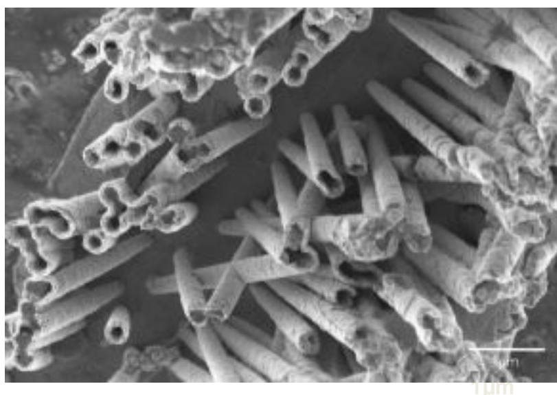
Figure 1. FEG-SEM micrograph of the as-deposited Co-Pt nanotubes.
