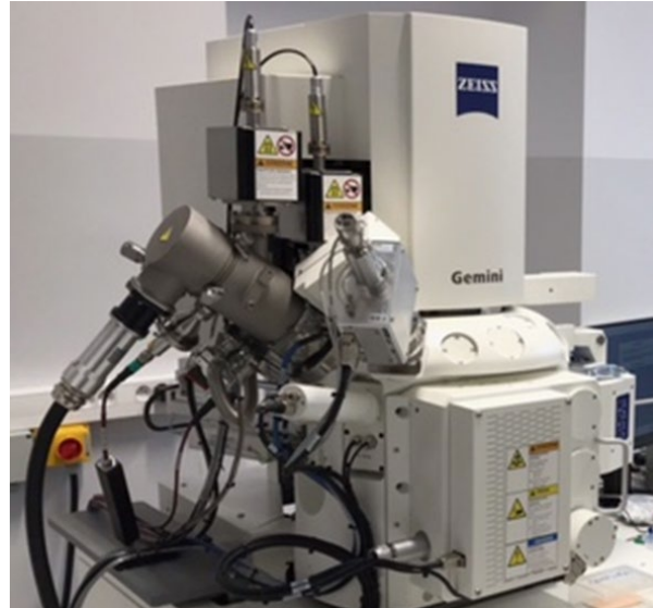
Fig. 13. Example FIB-SEM Crossbeam 350 dual-beam device (ZEISS)
