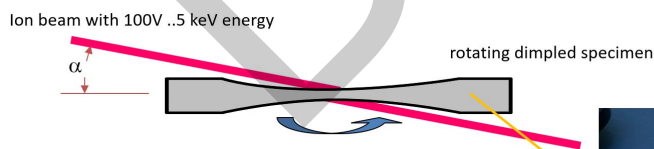
Fig. 6. NanoMill 1040 (Fischione) - ultra-low energy, concentrated ion beam device for producing the highest quality samples for TEM, free from preparation-induced artefacts (post-FIB processing)
