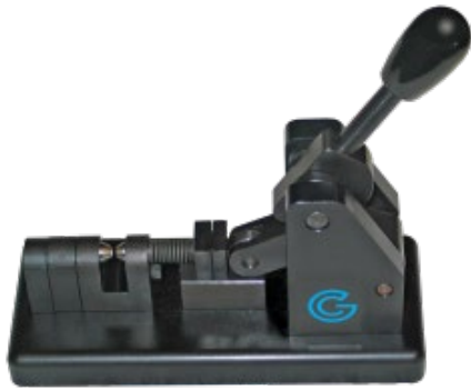
Punching of 3mm discs
