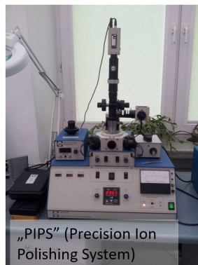
Fig.7. TEM specimen preparation final thinning, ion milling
