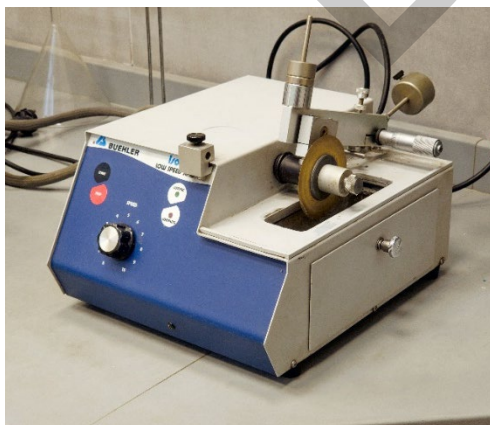
Sawing a slice of about 1 mm thickness
