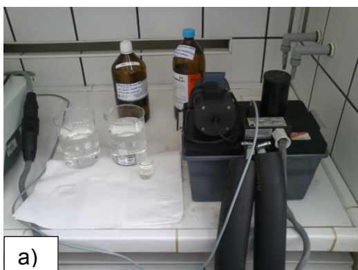
Fig. 5. Electropolishing unit (a), and a scheme of a twin-jet electropolishing apparatus (b).
