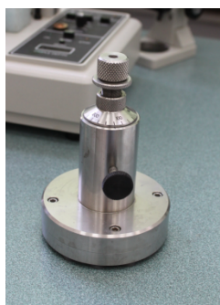
Fig. 3, Disc grinder, which allows to control remaining thickness of the specimen
