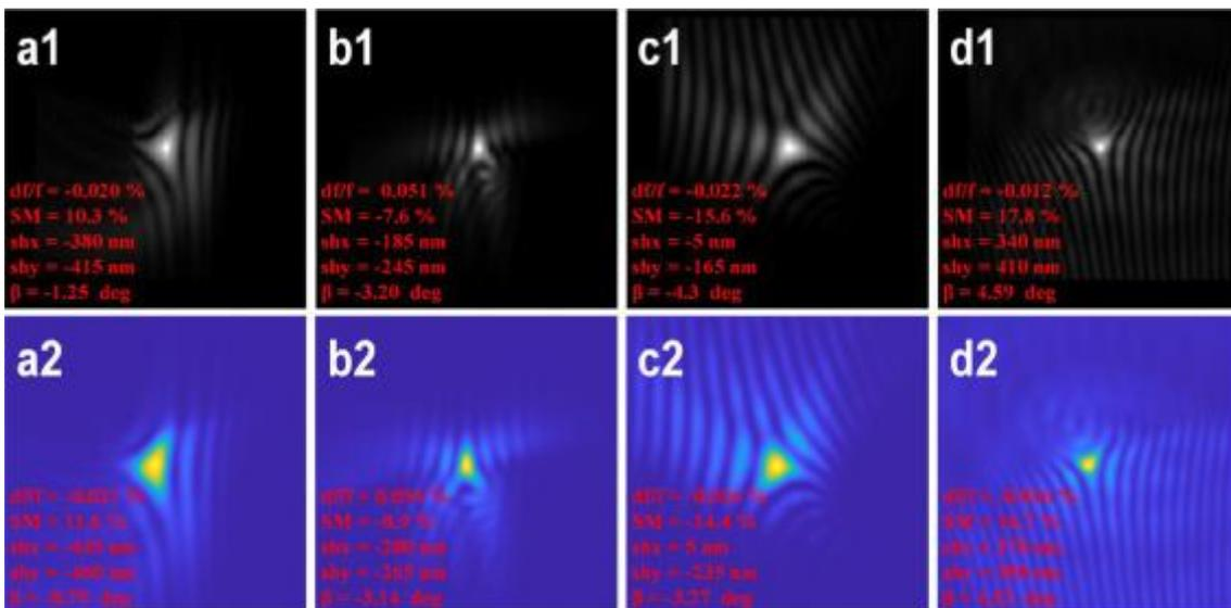
Figure 2: Adjustment parameters for the QSORT device derived from detector images using a neuronal network
