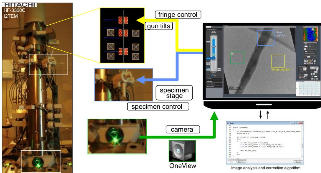
*Figure 2: Dynamic automation of the I2TEM microscope (TOU). Images are analysed continuously to determine specimen position and hologram phase. Feedback loops to specimen stage and gun-tilt coils ensure stability of experimental conditions.*
