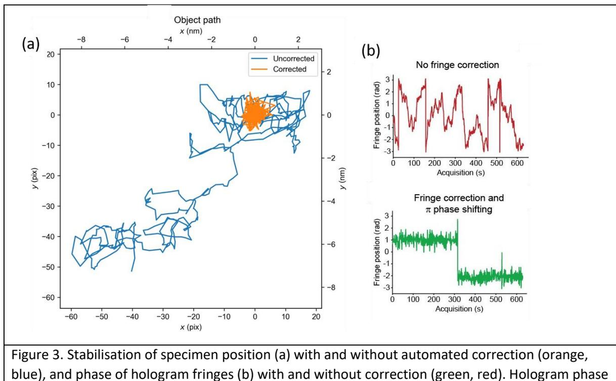
Figure 3. Stabilisation of specimen position (a) with and without automated correction (orange, blue), and phase of hologram fringes (b) with and without correction (green, red). Hologram phase
