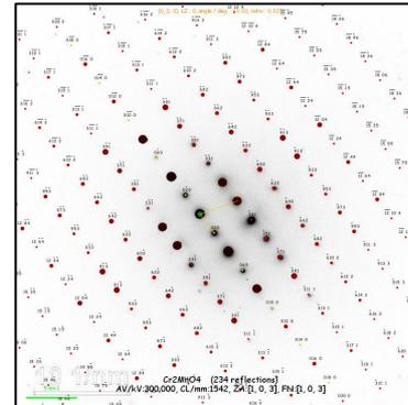
Simulated SAED of  $\text{Cr}_2\text{MnO}_4$ , superimposed on experimental one
