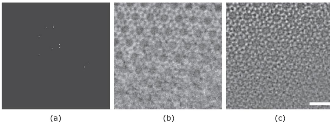
a) Example CBED pattern sequence, (b) iCoM reconstruction, and (c) SSB reconstruction for ZSM-5 using a cumulative electron dose of  $200 \text{ eA}^\circ 2$ . The scale bar for the phase reconstructions is 2 nm.
