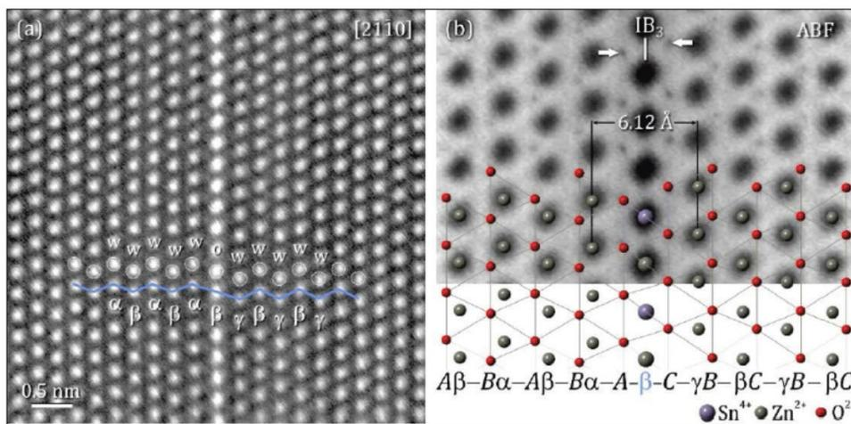
High-resolution STEM images of the Sn-rich IB in [21-1-0] projection. (a) HAADF-STEM image displaying a higher contrast for atomic columns along the IB-plane. Cation positions facilitate a direct identification of IB translation. (b) ABF-STEM image showing the positions of O-columns (weak dark dots).
