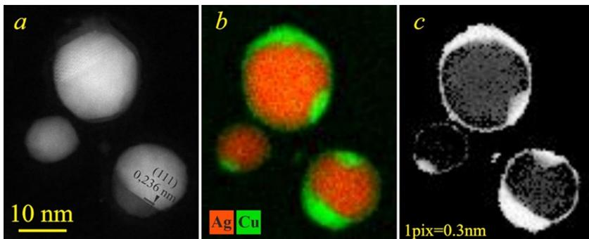
HAADF STEM image of the Ag-Cu binary nanoparticles at 300°C (a), corresponding EELS composite map of Ag and Cu (b), and Cu relative composition map (c).
