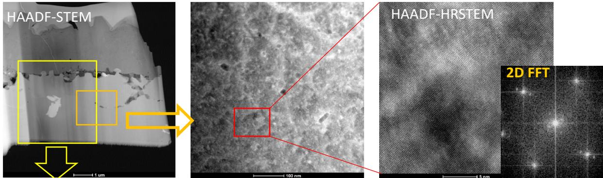
High-resolution TEM analysis of strengthening precipitates and a layer of scale after oxidation for 25 kh in steam
