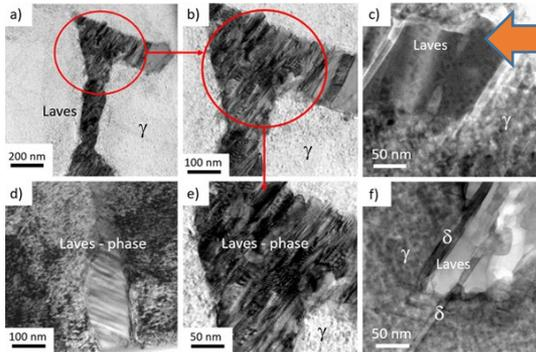
Decomposition of the Laves Phase in the Fusion Zone of the Inconel 718/ATI 718Plus<sup>®</sup> welded joint during isothermal holding at a temperature of 649 °C
