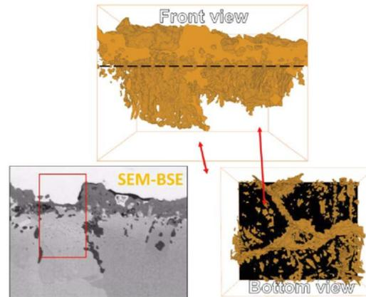
FIB-SEM tomographic reconstruction of oxides in the near-surface area of ME16 superalloy oxidized for 1000 hours at 730 °C.
