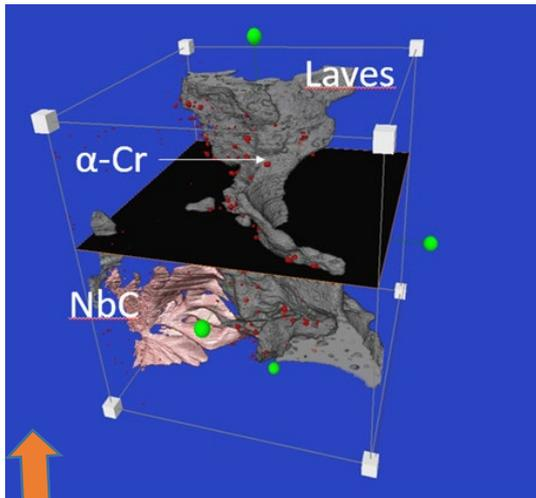
3D visualization of the tomographically reconstructed volume of 2.94 μm<sup>3</sup> of the IN718/718Plus weld area heat-treated for 50 h at 649 °C, containing the Laves phase precipitate and primary carbides of the welded joint. The voxel size: 1.5 x 1.5 x 3 nm
