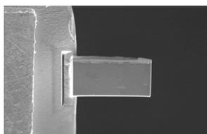
**Stage 7:** View of the mesh with the lamella attached.
