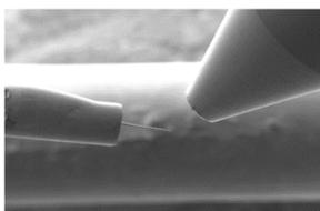
**Stage 8:** The stage of final thinning of the lamellae.
