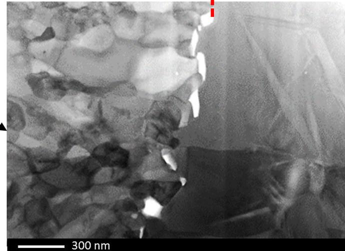
Magnification of **oxide scale-coating interface**
