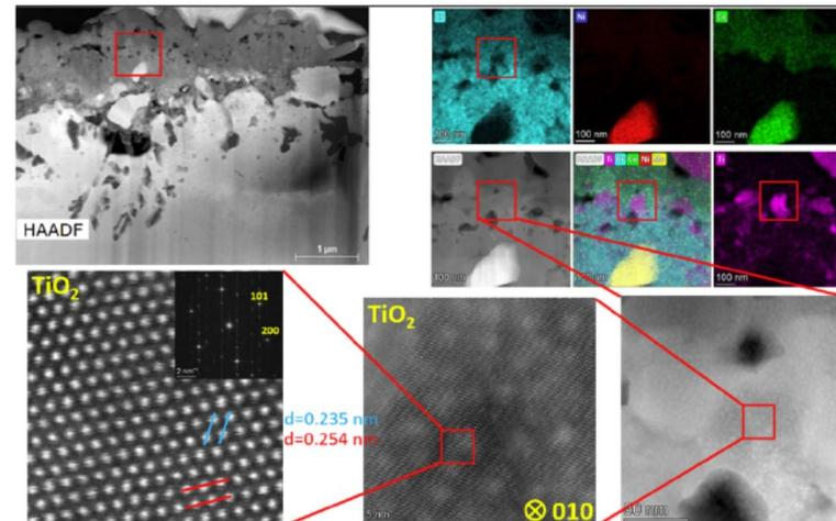
HRSTEM-HAADF/EDXS analysis of rutile at the interface of Co- and Cr-rich parts of the oxide scale.
