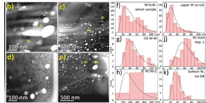
a) HAADF-STEM overview micrograph, with marked GBs (yellow lines) and regions of BF-STEM insets (white squares): b) bubbles at the W-W GB; c) bubbles outside the main implantation zone are limited to GBs (yellow arrows); d) He bubbles in the W grain outside main implantation zone, near sample surface; e) large elongated bubbles on inclined W|W<sub>2</sub>C interface (arrows mark upper and bottom contact).
