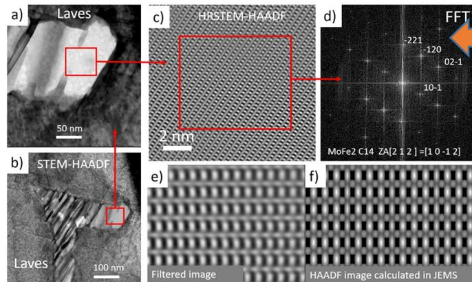
HRSTEM analysis of the Laves phase from the weld area of the IN718/718Plus welded joint after annealing for 50 hours at a temperature of 649 °C.
