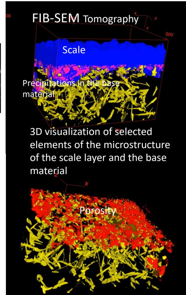
3D visualization of selected elements of the microstructure of the scale layer and the base material
