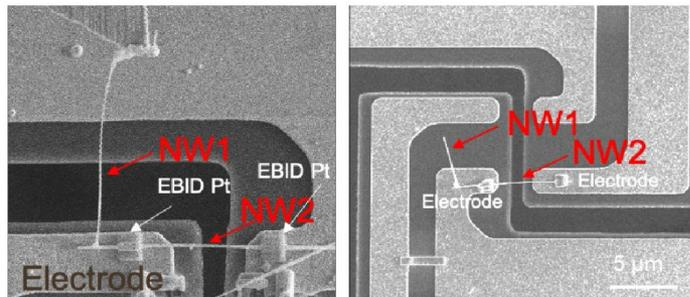
Specimen transfer to MEMS devices for *in-situ*
