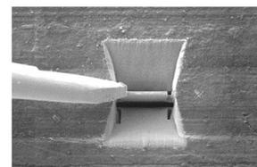
**Stage 3:** Welding the needle to the pre-cut lamella for pulling it out.
