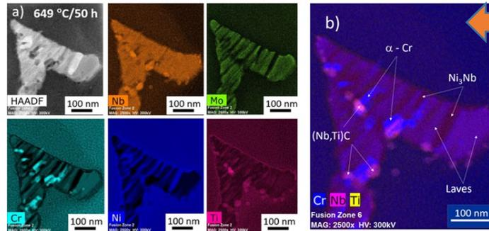
Qualitative STEM-EDX maps of the distribution of selected elements from the Laves phase area in the weld of the IN718/718Plus weld joint subjected to annealing after the welding process for 50 hours at a temperature of 649 °C.
