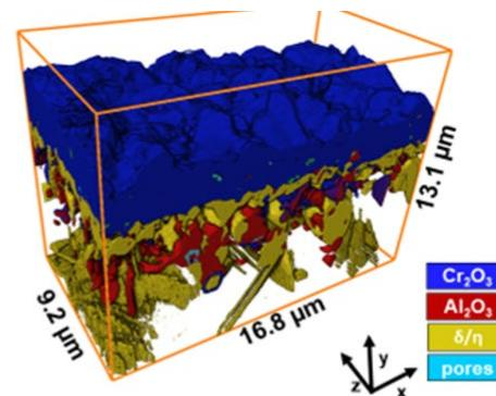
3D imaging of the microstructure elements of the base material and the scale on the surface of the 718Plus nickel superalloy sample.
