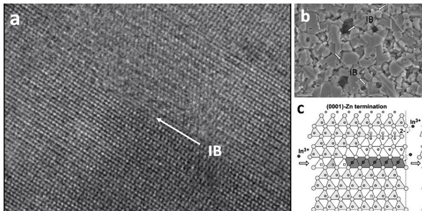
a) In-situ excerpt from movie showing a sequence of formation of the IB in  $\text{In}^{+3}$  doped ZnO. (b) IB's in  $\text{In}^{+3}$  doped polycrystalline ZnO. (c) The structure of the IB.
