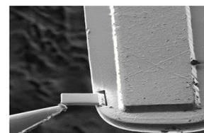
**Stage 6:** The stage of fixing the lamellae on the grid.
