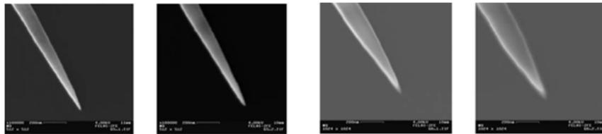
Sample prepared for TEM tomography from Allvac 718Plus nickel-based superalloy - *Internal cooperation with TU Graz in the frame of ESTEEM3.*
