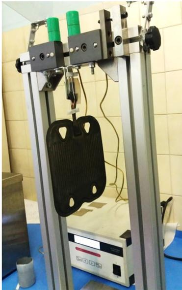
EPD adapted to a 3-electrode set-up
