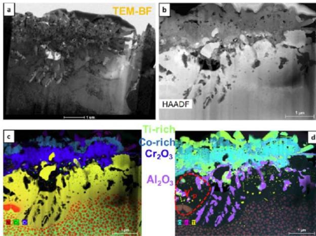
Lamellae of the near-surface area of ME16 superalloy oxidized for 1000 hours at 730 °C. a) TEM-BF image of the lamellae; b) STEM-HAADF image of the lamellae; c) Compositional STEM-EDXS elemental distribution map of Ni, Co, and Cr in the lamellae; d) Compositional STEM-EDXS elemental distribution map of O, Al, and Ti in the lamellae.
