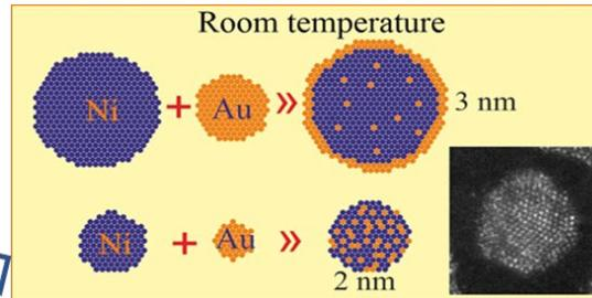
Size evolution of the solid-state miscibility gap in Au-Ni phase diagram.
