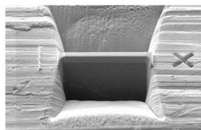
**Stage 2:** Pre-cutting of the lamellae
