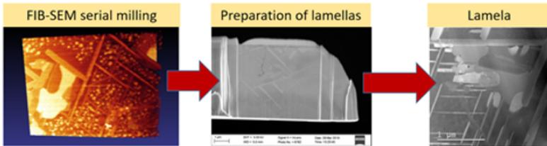
Correlative multiscale electron microscopy, 3D FIB-SEM tomography with detailed TEM investigation - targeted sample removal from analysed volume.
