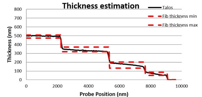
The thickness estimated (solid black line) is in a good agreement with that estimated by analysing the imaged acquired on the FIB (dash red lines) profile view.
