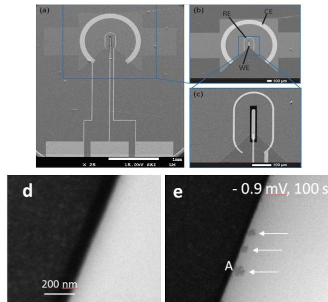
SEM micrograph of three electrode chip system for LC TEM (d) Work electrode before, and (e) after applying potential of  $-0.9 \text{ mV}$  for  $100 \text{ s}$ . The nucleation of Ni nanoparticles can be observed.
