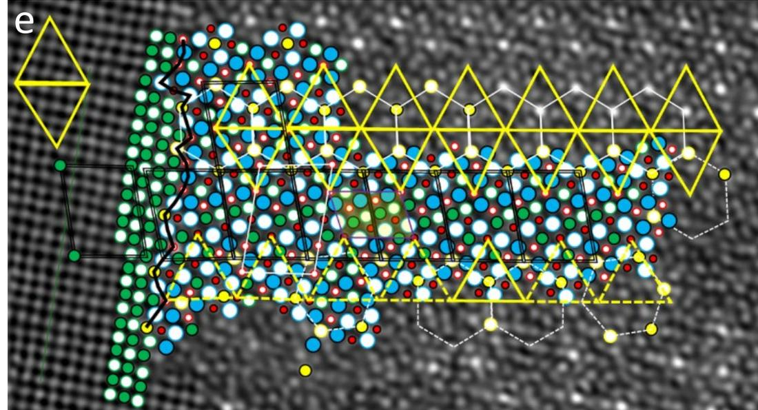
Fig (a) shows longer precipitates in the air-cooled and artificially aged samples both in the matrix and dispersoids, (b) shows finer precipitates on the dispersoids and the matrix in water-quenched and artificially aged samples, (c) shows larger precipitate free zones in air-cooled sample and (d) shows almost no precipitate free zones, (e) shows overlay of atoms in a defective secondary Q' precipitate
