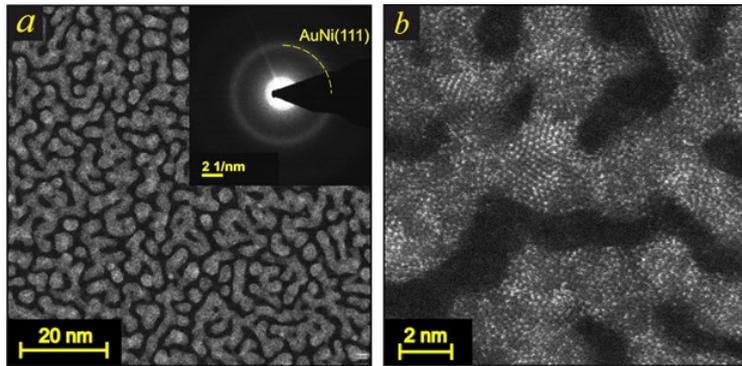
HAADF STEM image of the Au-Ni nanostructures with a size of 2 nm at room temperature and the corresponding EDX component distribution maps
