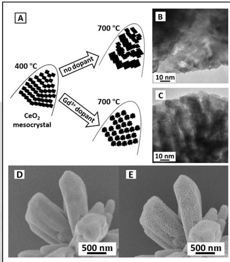
Stability of the architecture in soot combustion
