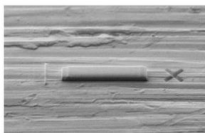
**Stage 1:** Selection of the area to cut out the lamellae (ROI) and place for deposition of the Pt layer.
