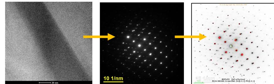
Simulated SAED of  $\text{Mn}_2\text{CoO}_4$  superimposed on exp. one [ZA 301]
