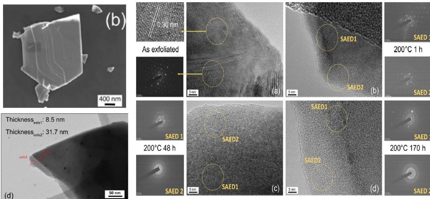
HRTEM images and related SAED patterns of the: (a) as exfoliated SnSe<sub>2</sub> flake; (b) 1 h; (c) 48 h; (d) 170 h annealed SnSe<sub>2</sub> flakes in air at 200 °C.
