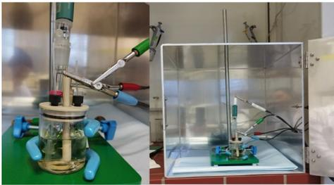
**Step 2:** *Ex-situ* electrochemical characterization using MEMS chips
