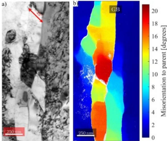
Misorientations in precipitate free zones of a compressed Al-Mg-Si alloy
