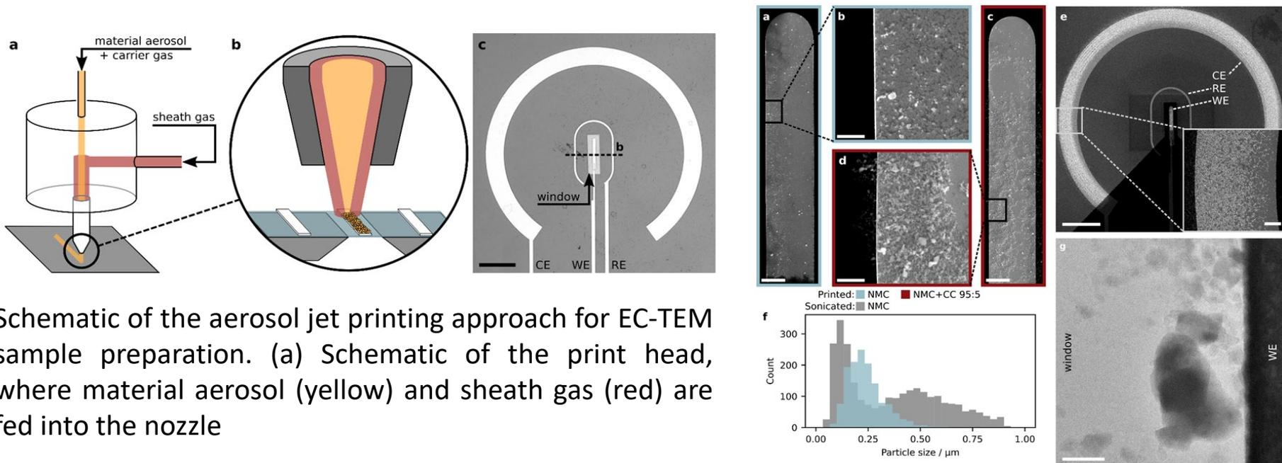
Schematic of the aerosol jet printing approach for EC-TEM sample preparation. (a) Schematic of the print head, where material aerosol (yellow) and sheath gas (red) are fed into the nozzle
