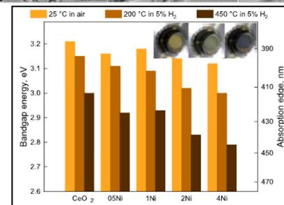
Bandgap energies for bare CeO<sub>2</sub>-R and Ni/CeO<sub>2</sub> catalysts containing 0.5–4 wt% Ni in air at 25 °C and 200 °C and 450 °C in 5% H<sub>2</sub>/N<sub>2</sub> atmosphere. Inset shows the 2Ni catalyst at mentioned temperatures and atmospheres.
