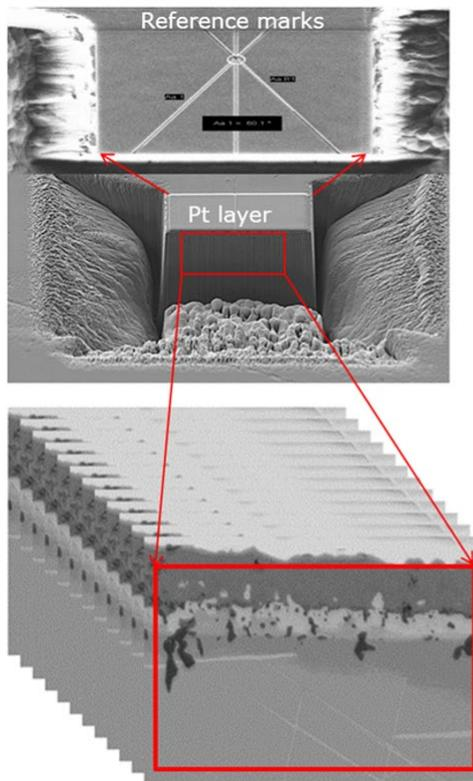
Tomographic series of SEM-BSE images from the area of the substrate material and the scale layer of the oxidized nickel superalloy sample.
