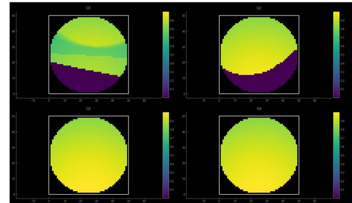
calculated EDX shadowing for each detector
