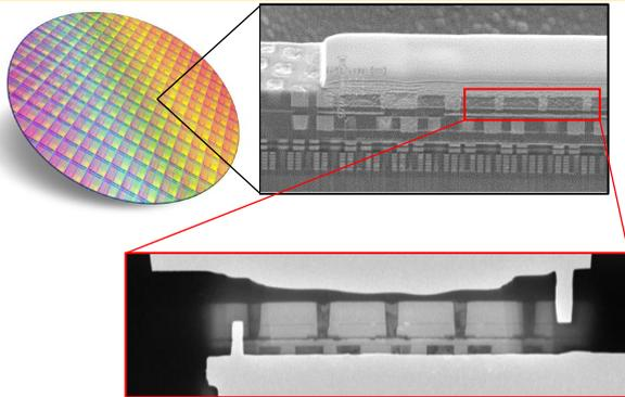
MIM nanocapacitors (STMicroelectronics)
