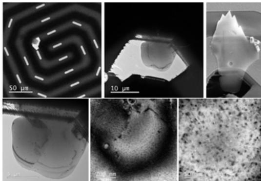
The aluminium lamellae preparation for in-situ heating in TEM. BF-TEM images and a SEM image (top right) of an aluminium lamella attached to a DENS chip for in-situ heating in TEM. Results from NTNU TRO.
