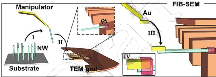
Preparation for *in-situ* electrical measurements on nanowires
