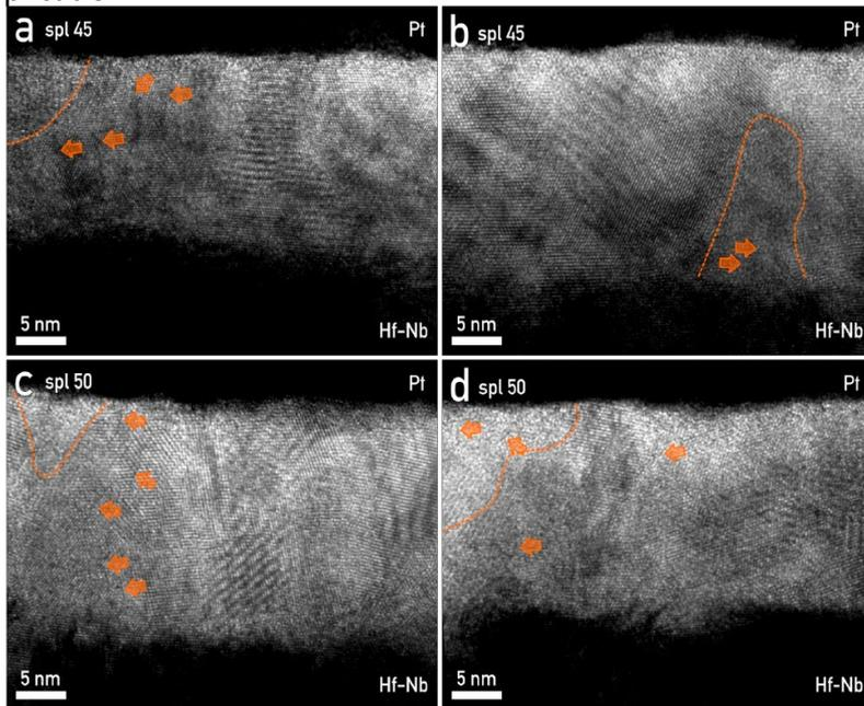
HR-TEM micrographs of Hf–Nb oxide layer. (a,b) Sample Hf-45 at.% Nb, (c,d) sample Hf- 50 at.% Nb. Crystalline  $\text{HfO}_2$  was sporadically interrupted by amorphous  $\text{Nb}_2\text{O}_5$  regions (outlined with a dashed orange line). The conductive filaments emerging from metal layers are marked by orange arrows
